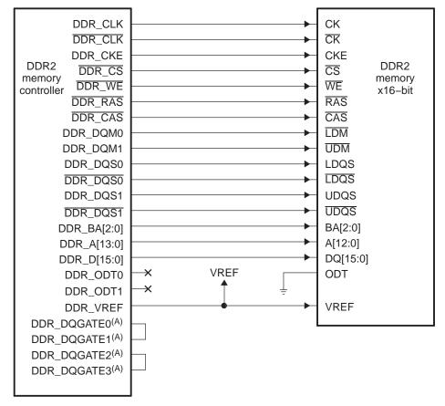
Figure 18. Connecting to a Single 16-Bit DDR2 SDRAM Device
